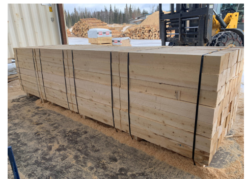
Pipe skids, like those shown here side-by-side at Seaton Forest Products, hold pipe sections in place while they are being welded together.
